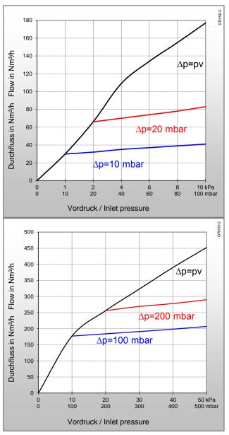
Example flow rate type: GRV50-VA G2RH F/F. Values for other connections on request.
