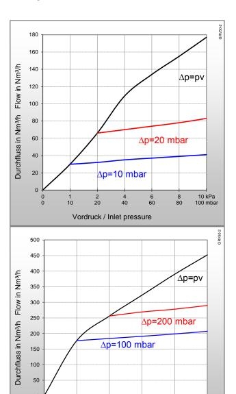
Example flow rate type: GRV50 G2RH F/F. Values for other connections on request.
