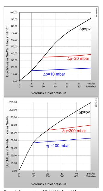
Example flow rate type: GRV32-VA G1 1/4 IG. Values for other connections on request.
