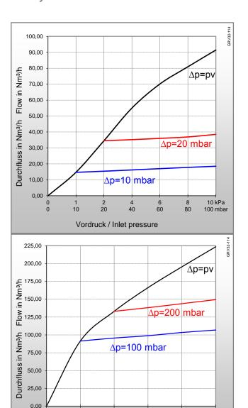
Example flow rate type: GRV32 G1 1/4RH F/F. Values for other connections on request.
