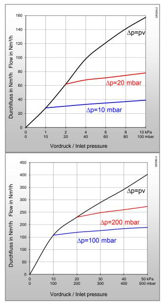
Example flow rate type: GRS50-VA G2RH F/F. Values for other connections on request.
