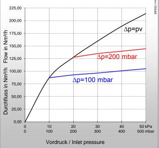
Example flow rate type: GRS32-VA G1 1/4RH F/F. Values for other connections on request.
