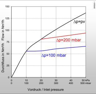
Example flow rate type: GRS25 G1RH F/F. Values for other connections on request.
